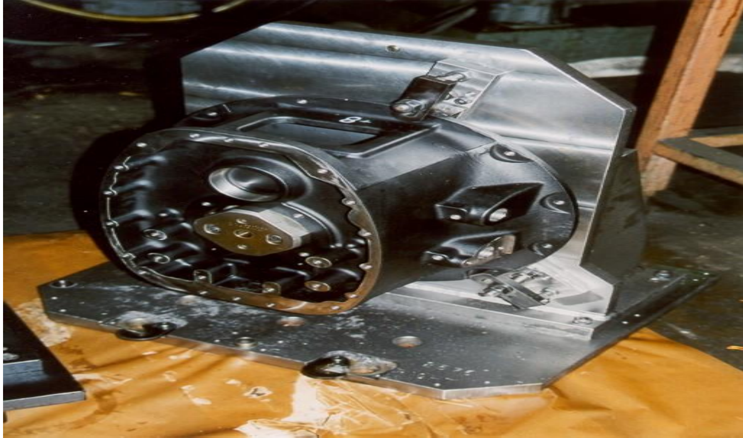
Example of a part mounted on a pallet
