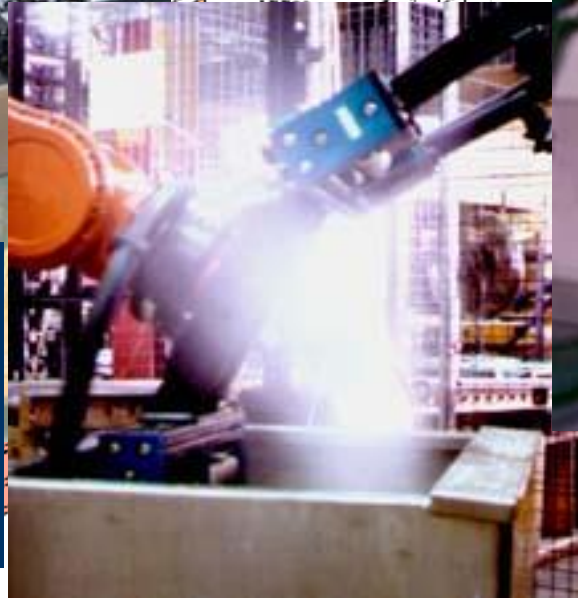
Holding a cast wheel while it is being cleaned with live steam.
